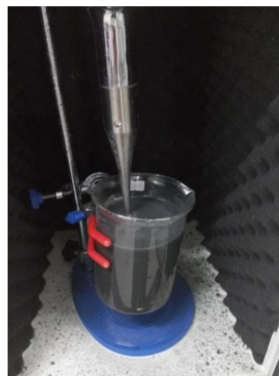
Fig. 2: Ultrasonic treatment of wounded maize seeds with the addition of emery grits
